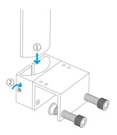
**Step 3**Slide the X-Bracket onto the Sliding Rail, align the hole with the Slide-in economy T-nut, then tighten down the screw.
