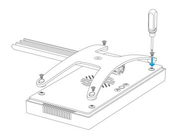
**Step 5**Guide the Sliding Rail onto the Formed Arm, and tighten the screw to lock it in desired position.
